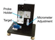
3. Select a  $SHD\ A$  (aluminum) or  $SHD\ D$  (brass) target and insert it into the load cell as shown. **Note:** Inspect the targets before installing. To prevent damage to the PosiTector  $SHD\ D$  probe tip, the  $SHD\ D$  (brass) target is designed to be dented during testing and will periodically need to be replaced. The  $SHD\ A$  (aluminum) target will not be dented during testing and should be replaced if there is any damage to the top surface.
